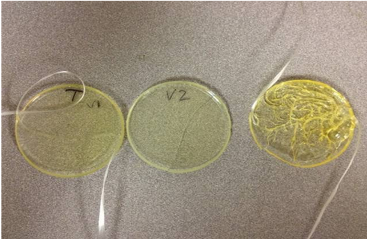
Figure 15: Acrylate (right) versus Methacrylate (left and center)
